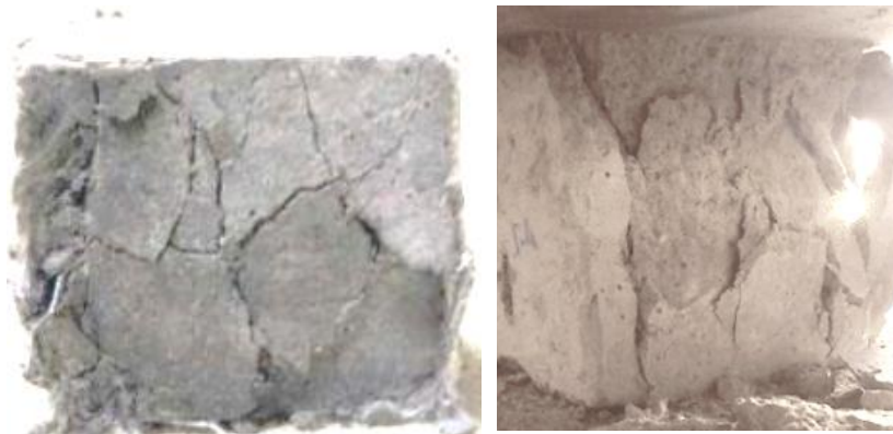
Fig 8. Failure mode of the mortar samples
