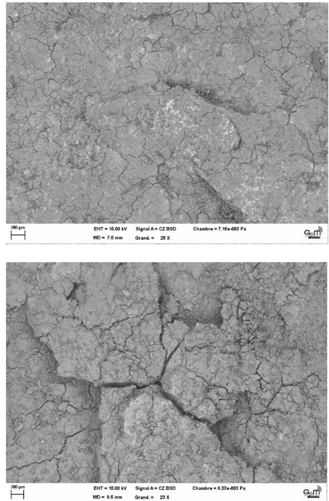
Fig. 5. SEM photomicrograph after immersion in EXCO solution for different alloys.
