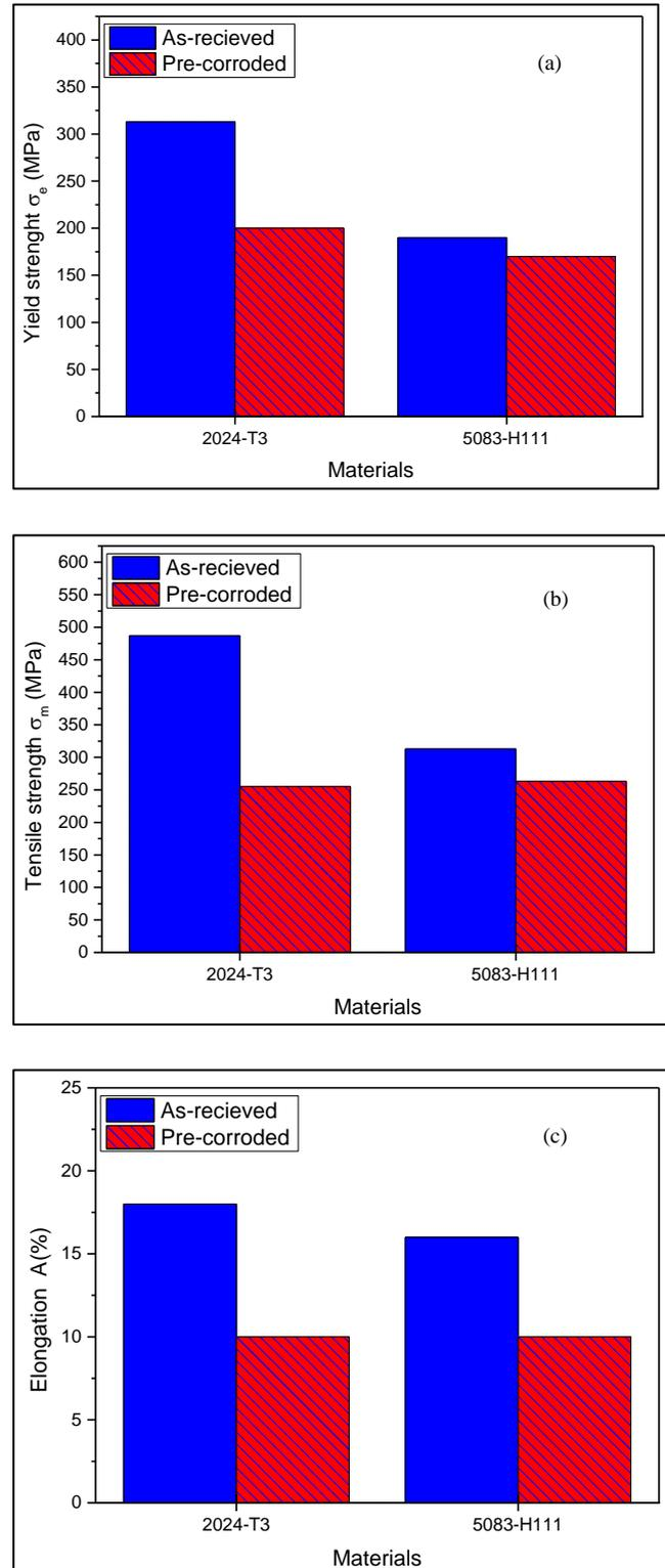
Fig. 2. Residual strength properties (a) yield strength  $R_e$ , (b) tensile strength  $R_m$  and (c) Elongation A% for the different materials.
