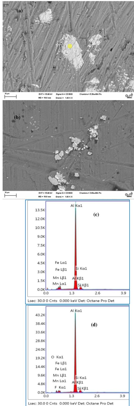
Fig. 3. SEM photomicrographs and EDX spectra showing the microstructure of : a) AA5083-H111, b) AA2024-T3 before the chemical attack.
