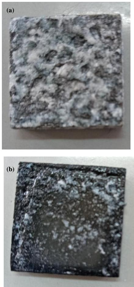
Fig.4. Degree of severity of corrosion for: a) 5083-H111, b) 2024-T3.
