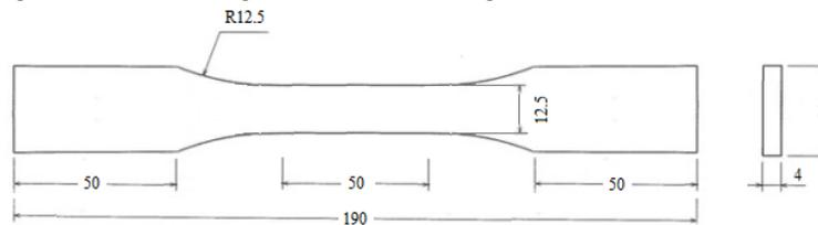
Fig. 1. Tensile test specimen
